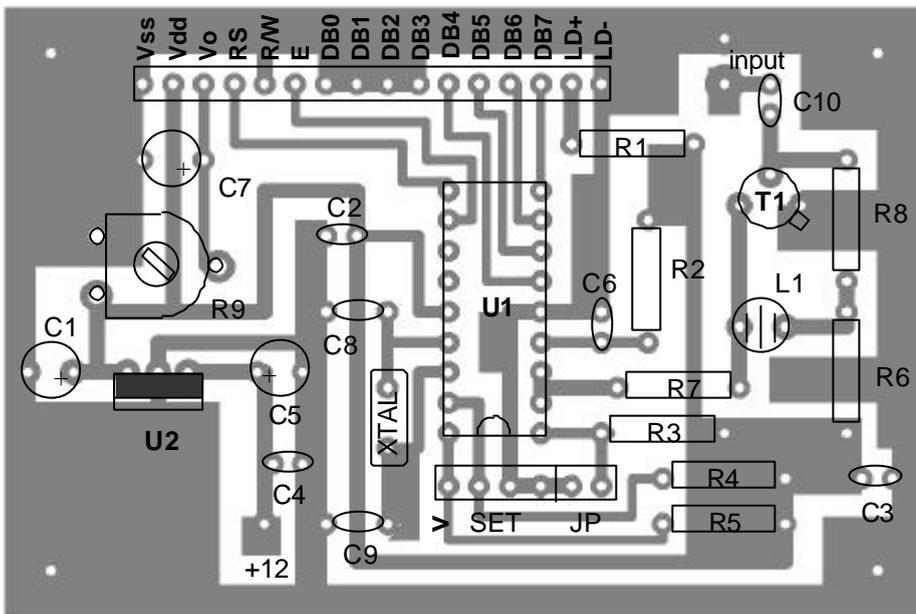
The assembly is done on a single sided PC board measuring 76 x 51 mm. On the board are placed also a female 16 pin connector, 2.5 mm spacing, to match the LCD module and a male 6 pin connector to link the two push buttons and the JP jumper. The components placement is shown clearly in the picture, and the assembly is very simple, due also to the small number of parts.
