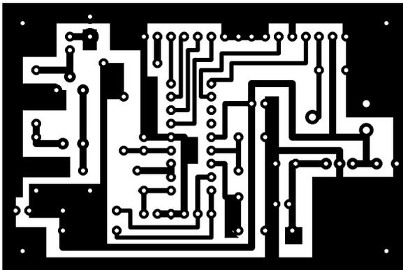
The 1:1 PCB may be reproduced in several ways. I suggest to copy it on a transparent using a good quality laser photocopier, or by means of a scanner and an inkjet printer. Next you may employ a usual photo etching technique. I may provide the master in CIRCAD format to those who are interested.
